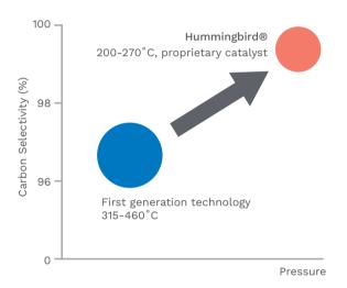
Hummingbird is a second generation, low-cost process for dehydrating ethanol to ethylene. The technology uses a proprietary heteropolyacid (HPA) supported catalyst, operating at a lower temperature, higher pressure, and higher selectivity than first generation processes.
