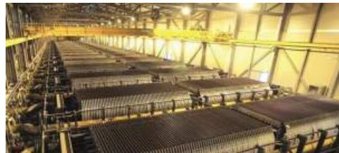
BICHLOR™ is a modular electrolyser comprising a series of discrete modules consisting of anode, membrane and cathode.
