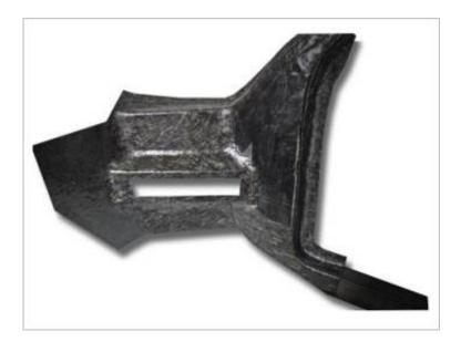
The technology is based on a one-step "carbon fiber bobbin to preform" concept, utilizing *TENAX* Binder Yarn, which combines carbon fibers with a binder resin. The yarn can be processed by random fiber placement for isotropic behavior, and by aligned fiber placement in those areas, where higher mechanical performance is required. Both technologies - random and aligned fiber placement - can be combined to meet specific mechanical and/or cost needs.
