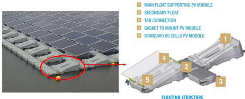
Photo of a similar floating solar installation (left) and diagram of Ciel et Terre's floating platform (right)
