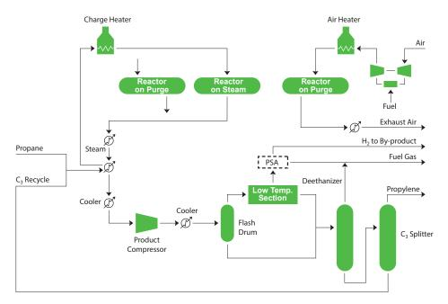
The diagram shown is for the production of propylene. For isobutylene production, the deethanizer and  $C_3$  splitter are replaced by a depropanizer. A deoiler is also included to reject a small amount of  $C_4$ s
