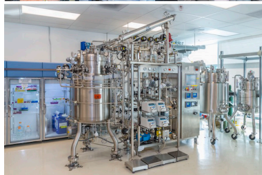
Top: Lygos co-founders with Todd Pray, head of the ABPDU. From left: Leonard Katz, Pray, Eric Steen, Jeffrey Dietrich, and Jay Keasling. Bottom: Fermenter used in the scale-up of malonic acid. (Credit: R. Kaltschmidt/Berkeley Lab)
