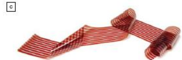
Figure 1. (a) Schematic layout of the function of a typical organic solar cell. (b) Chemical structures of typical donors and acceptors. (c) Photograph of reel-to-reel-fabricated organic solar cells. The active layer of the solar cells is a P3HT/PCBM blend. Note: P3HT is poly(3-hexylthiophene), PCBM is [6,6]-phenyl-C61-butyric acid methyl ester, PEDOT is poly(3,4-ethylenedioxythiophene), PSS is poly(4-styrenesulfonate), and TCO is transparent conductive oxide.
