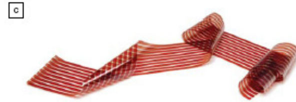
Figure 1. (a) Schematic layout of the function of a typical organic solar cell. (b) Chemical structures of typical donors and acceptors. (c) Photograph of reel-to-reel-fabricated organic solar cells. The active layer of the solar cells is a P3HT/PCBM blend. Note: P3HT is poly(3-hexylthiophene), PCBM is [6,6]-phenyl-C61-butyric acid methyl ester, PEDOT is poly(3,4-ethylenedioxythiophene), PSS is poly(4-styrenesulfonate), and TCO is transparent conductive oxide.
