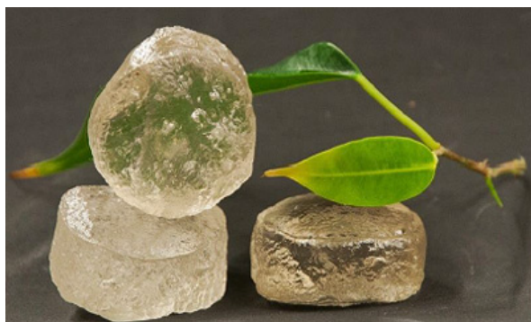
Versalis has produced bio-based rubber using bio-butadiene from its joint venture with Genomatica
