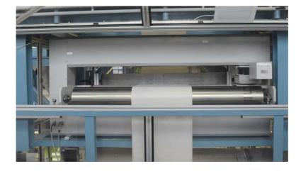
**Caption:** Evonik has started to operate a thin-film composites plant to coat membranes for use in organic solvent nanofiltration.
