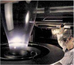
uniformly distributed. Monolayer or complex multilayer K-Resin<sup>®</sup> SBC films may be produced on cast film equipment as well as blown film equipment. The cast film process is well suited to K-Resin<sup>®</sup> SBC film because of the low level of wrinkles and excellent gauge control of the process. Producing blown film is more challenging, but does offer improved film properties.
