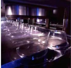
K-Resin<sup>®</sup> SBC sheet can be thermoformed using any of the common techniques, such as male or
