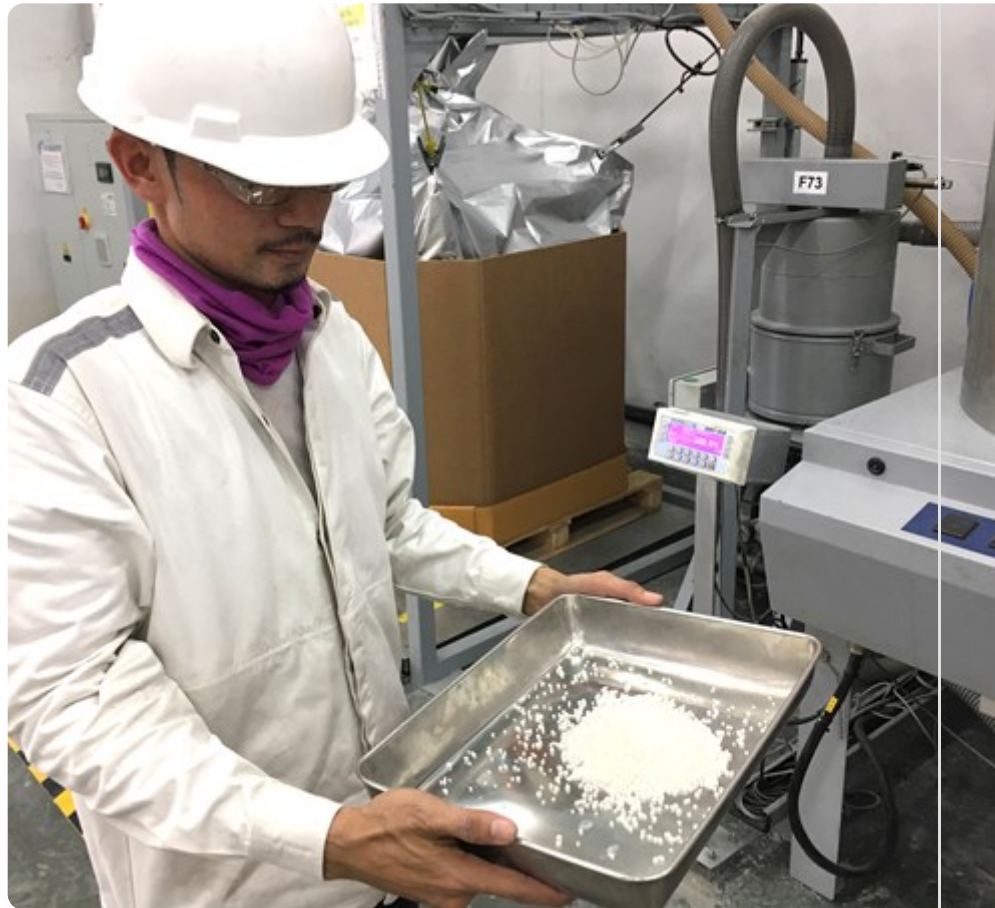
Quality inspection of Luminy® biopolymer pellets produced from Total Corbion PLA's pilot plant in Rayong, Thailand.
